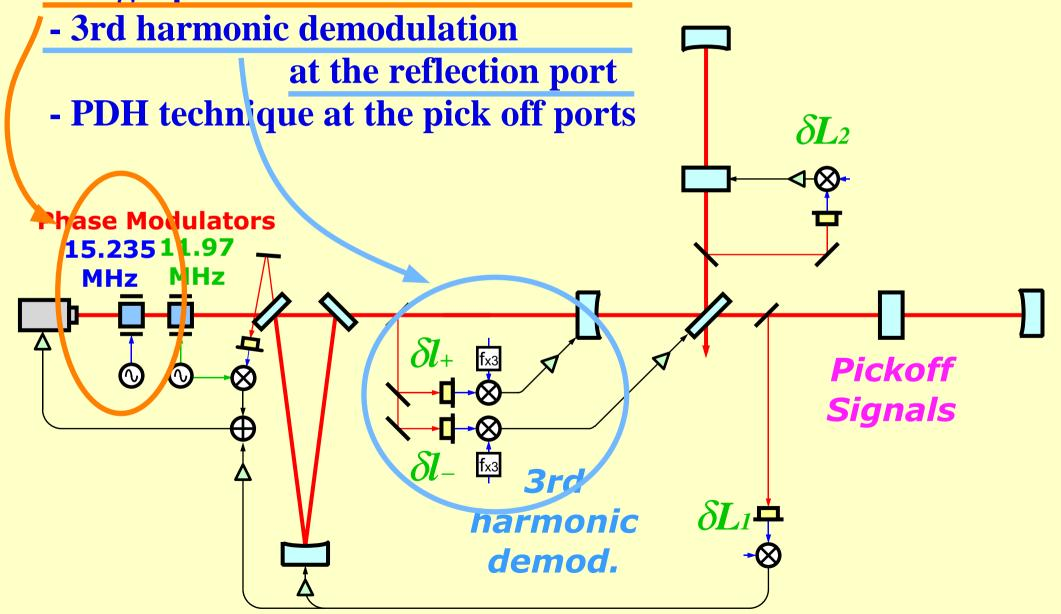
Based on the PDH technique and Schunupp modulation
