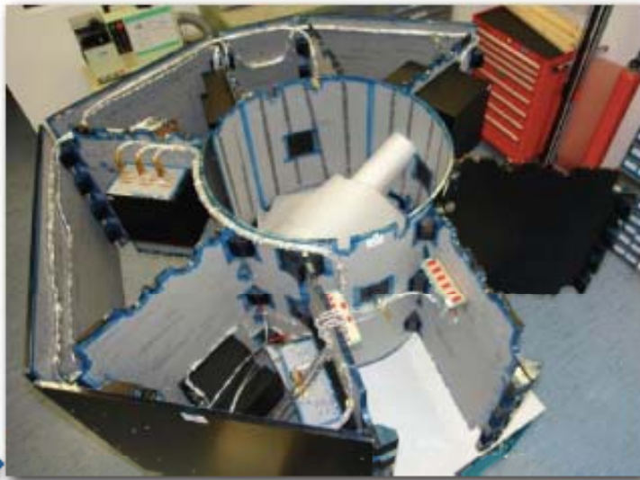
FM electrical harness check
